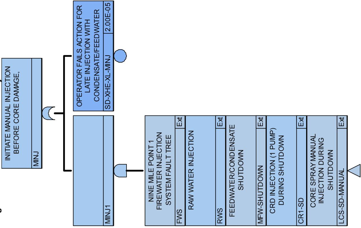
Figure A-5: Long Term Recovery after Successful Injection Fault Tree
